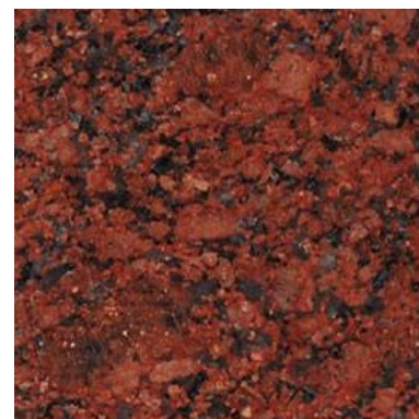
2. Existing Granite Cladding Colour: Red Granite
